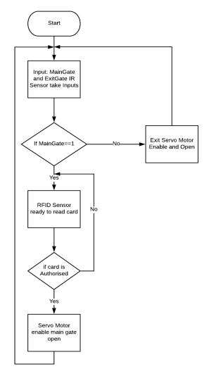
Fig. 2 system flow Diagram
